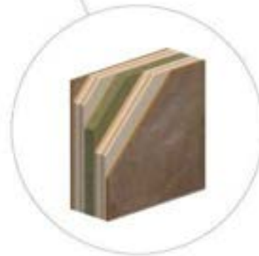
Load-bearing Internal Wall (625 mm)
