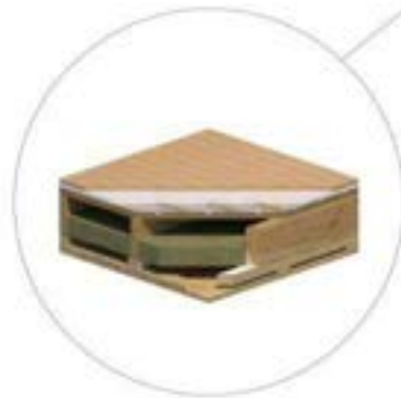
Floor Slab (385 mm)
